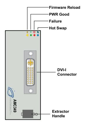
FIGURE 2. AMC349 Front Panel
