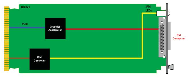
FIGURE 1. AMC349 Functional Block Diagram
